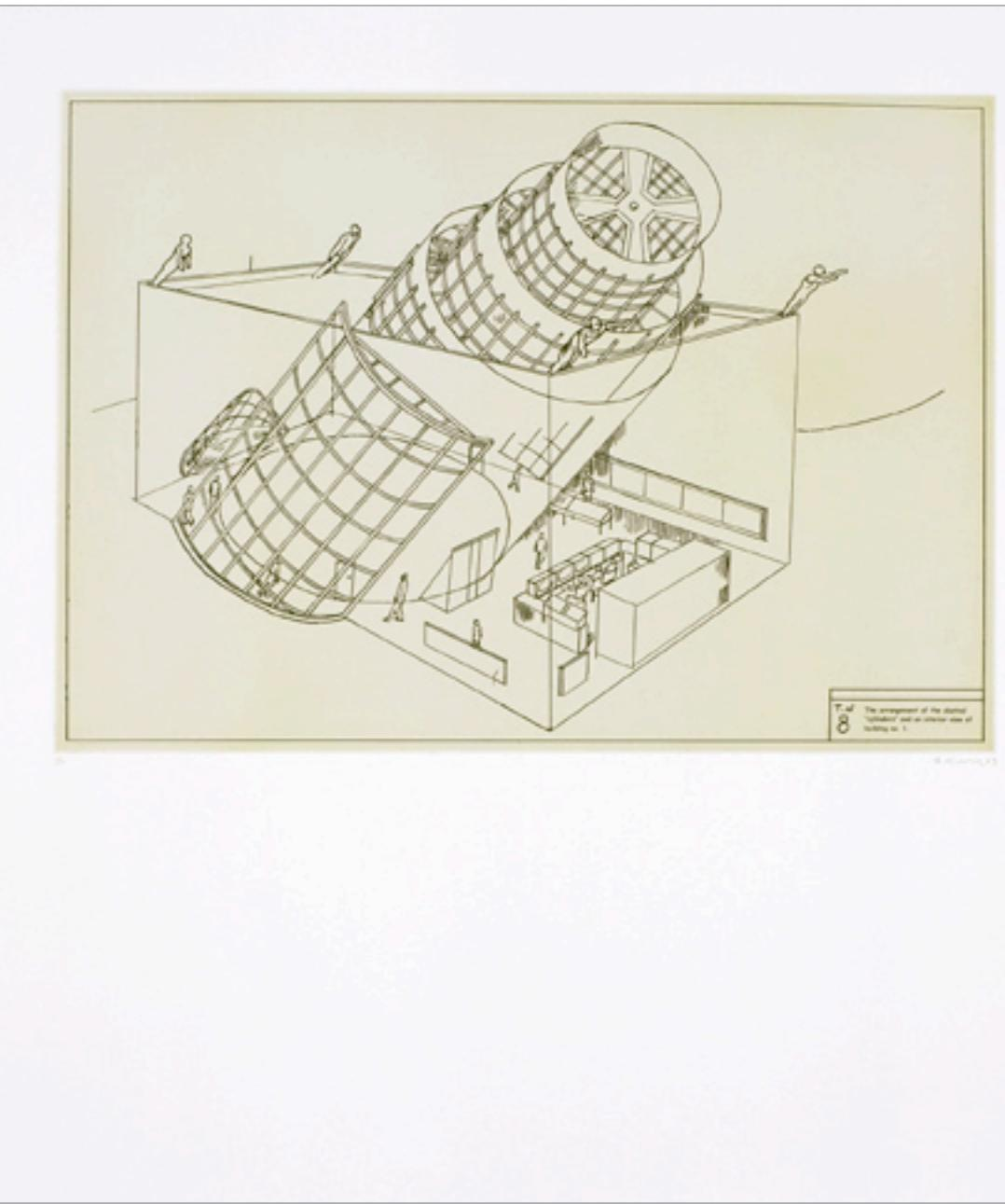
The arrangement of the slanted “cylinders” and an interior of building No. 1.
