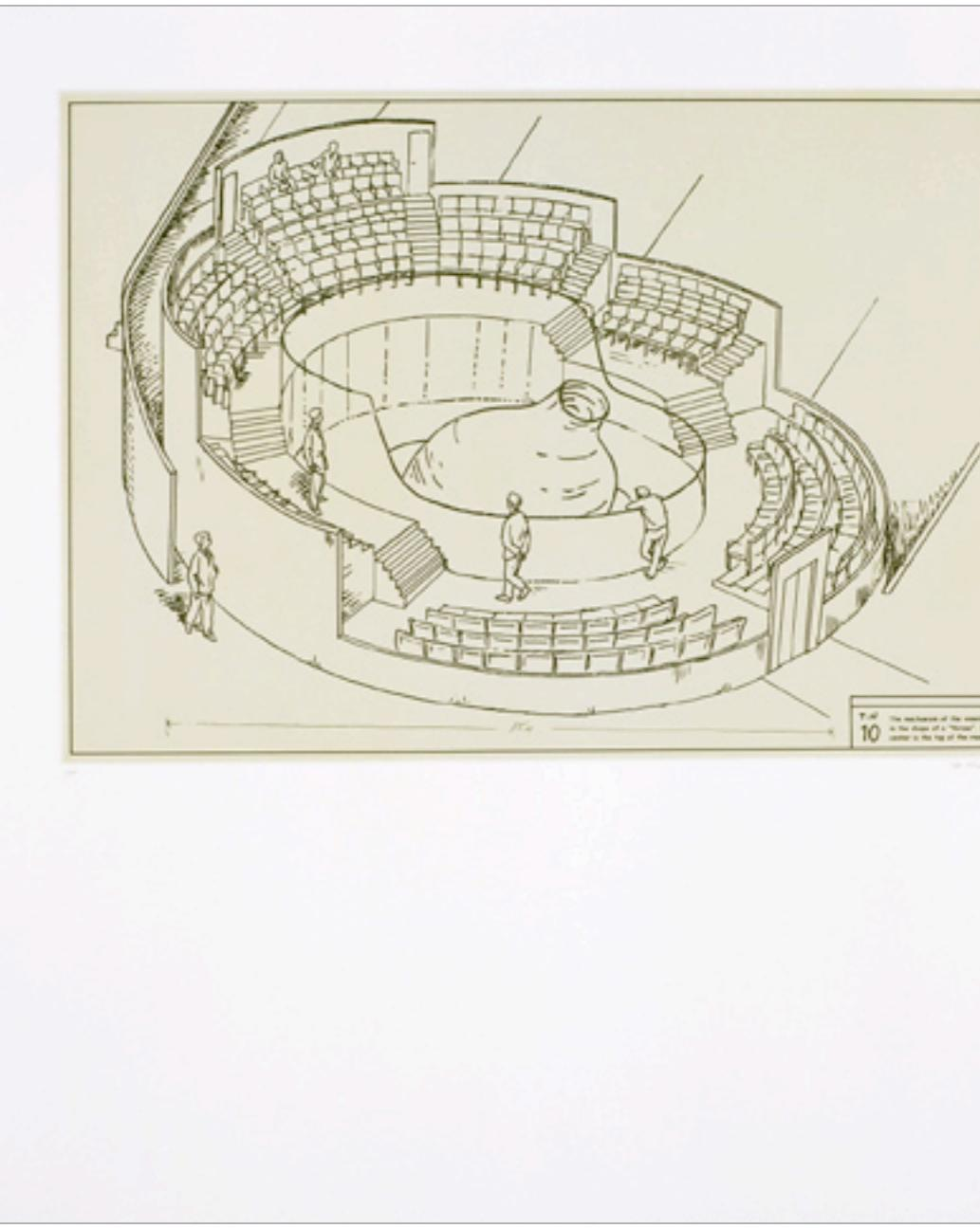
The structure of the viewing hall in the shape of a "throne". In the center is the top of the reservoir.
